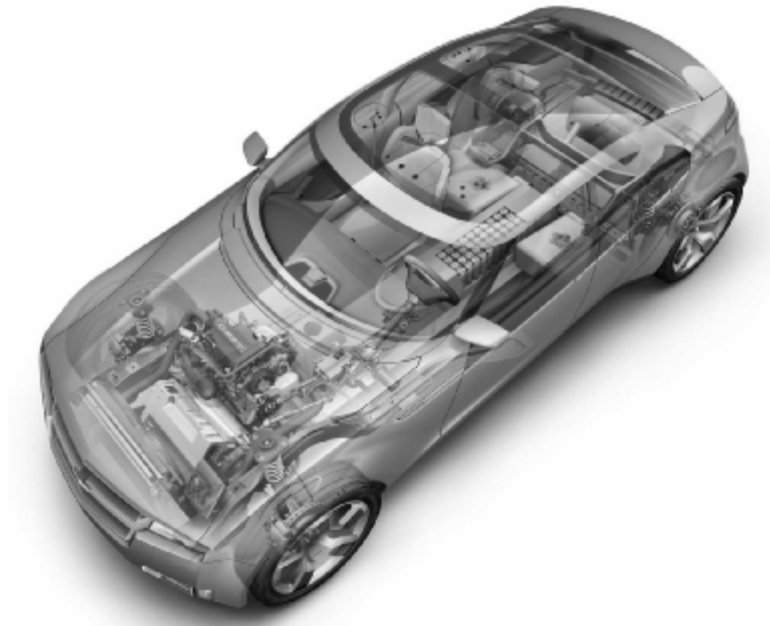
Illustration 10: Concept vehicle Chevrolet Volt: a one-litre three-cylinder turbo petrol engine turning at a constant speed produces current to recharge the batteries located in the transmission tunnel (Source: General Motors)
