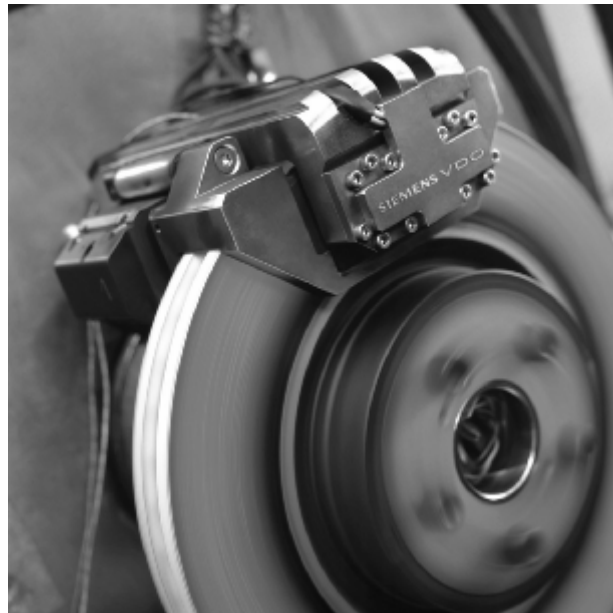
Illustration 16: An electronic wedge brake being tested (Source: Continental/Siemens VDO)
