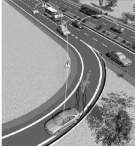
Illustration 21: Local 'car to car' communication (Source: CAR 2 CAR Communication Consortium)
